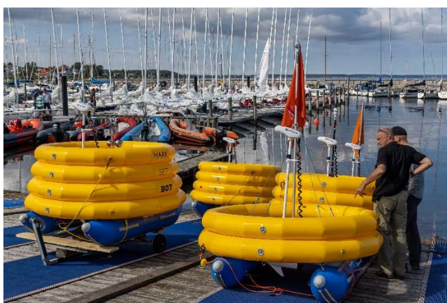
Launch of self-positioning marks with idle RIBs in the background.
