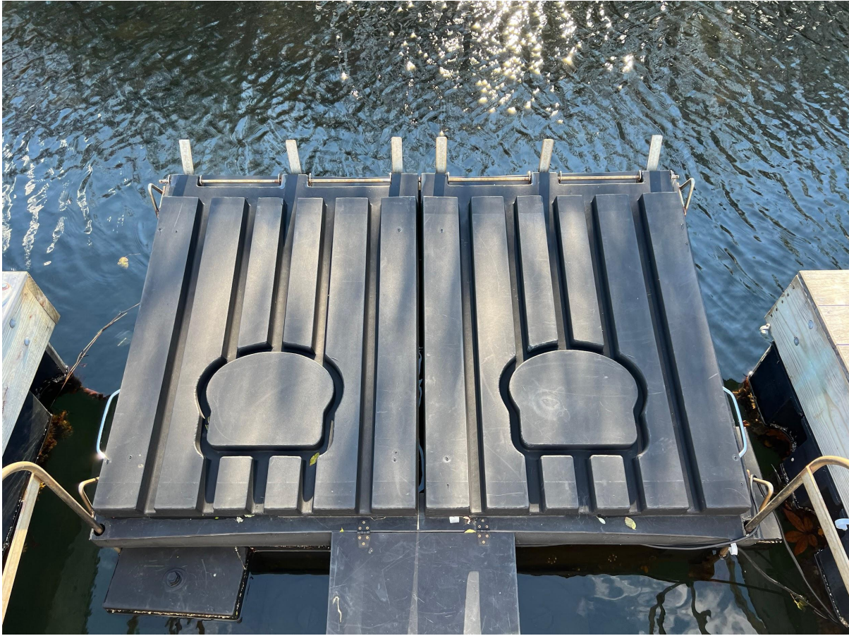
The marina trash skimmer not only collects debris, but oil slick from the water as well.
